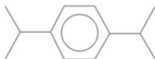
Figure 2. Structure of p -diisopropylbenzene (DIPB). The addition of cumene to propylene via further alkylation leads to this undesired byproduct (NIST 2011).
