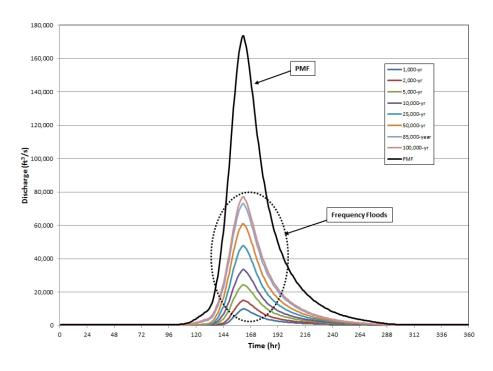
Figure 2.4.1-1. Example frequency flood hydrographs and relationship to the PMF
