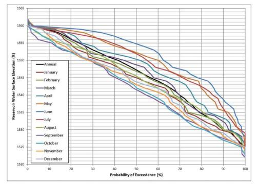
Figure 2.2.1.6-3. Example: Reservoir exceedance curves for each month, based on historical daily reservoir data, as initial reservoir water surface elevation ranges for frequency flood routings.
