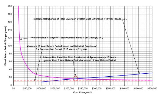
Figure 2. Identification of construction diversion flood base on costs, Dam R.
