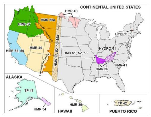
Figure 2.2.1.3-1. Generalized HMR series typically used to estimate PMP for Federal projects within the United States.
