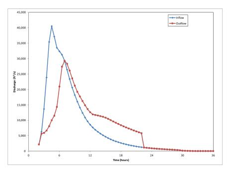
Figure 2.2.1.6-2. Example: Inflow and outflow hydrographs from reservoir routing.
