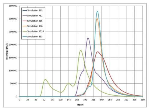
Figure 2.3.2-1. Example: Reservoir inflow frequency hydrograph variations based on a 1/10,000 AEP volume.
