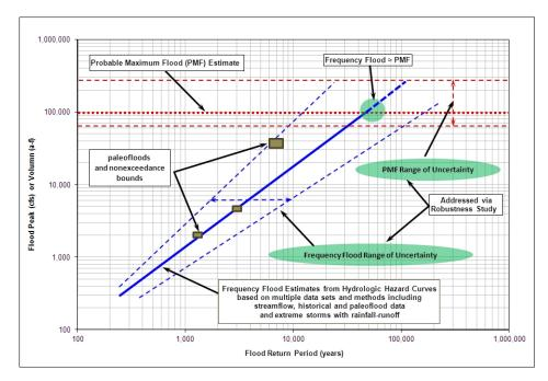
Figure 2.4.1-2. Generalized HHC schematic (relationship between the PMF and frequency floods).
