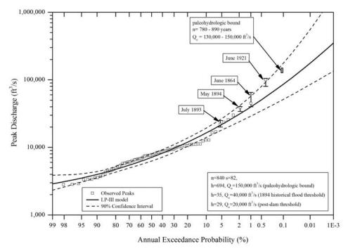
Figure 2.2.1.1-1. Example: Hydrologic hazard curve (with uncertainty) based on peak flows.
