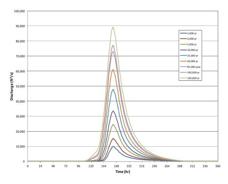
Figure 2.2.1.1-2. Example: Frequency flood hydrographs.
