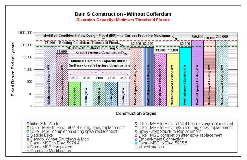
Figure 1. Diversion capacities during construction stages.
