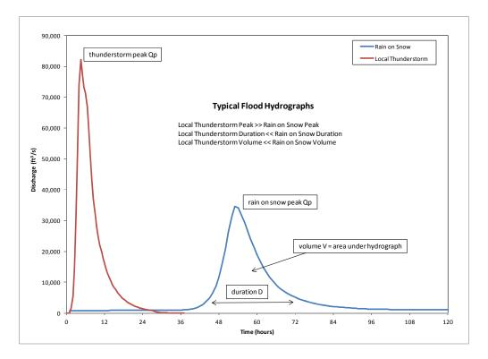
Figure 2.2.1-5. Example: Flood hydrographs showing typical shapes and peaks, volume, and duration relationships.
