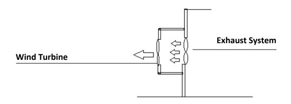
**Power Recovery on Exhaust Fan System**
