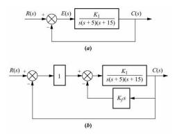
Design a feedback compensator to reduce the settling time by a factor of 4 while continuing to operate the system with 20% overshoot.
