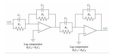
We are actually able to implement lag, lead compensators with passive circuits:
