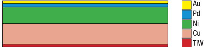
Cross-section of sputtered copper with plated ENEPIG
