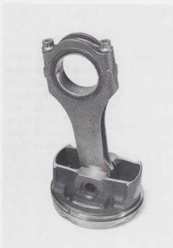
Ferrari S.p.A. Piston with Connecting Rod for Engine of the F1, 1990. Aluminum alloy and titanium. Mfr.: Ferrari S.p.A. Photo: Mali Olatunji
