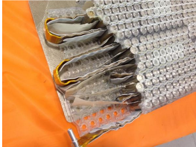
Figure 12. Tesla Model S and X battery module [28]
