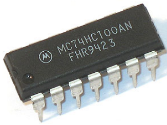
Figure 2. A typical digital logic integrated circuit, specifically one that could be used to implement most of the logic in the previous figure.
