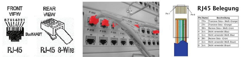
Figure 6: Ethernet RJ45 connector (with pin layout)
