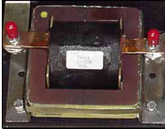
Fig. 37. Photo of the finished input inductor
