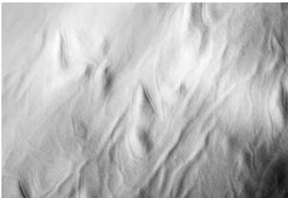
Figure 1: Plan-view TEM of \text{In}_{0.43}\text{Al}_{0.57}\text{As} on GaAs with a dislocation density of 1.4\text{E}6/\text{cm}^2 .
