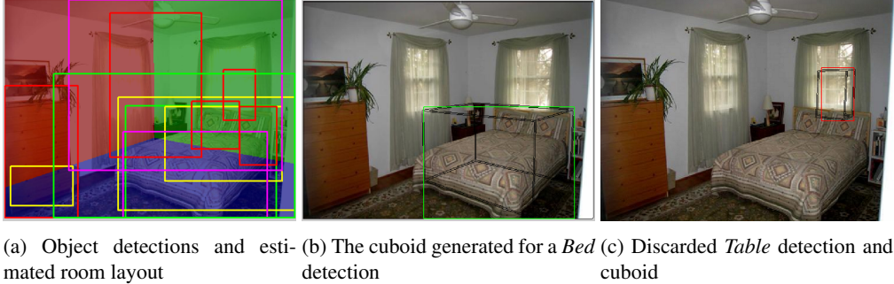
Figure 2: 3D cuboids are generated from object detections’ bounding boxes. Cuboids lying behind walls are discarded
