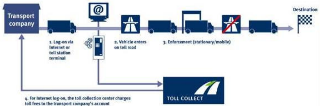
Figure 16: Truck Toll Collection – Manual booking (on the internet or at toll station terminal)
