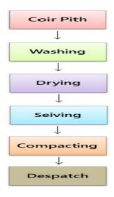
High electrical conductivity (EC) of coir pith is the major constraint in using it as growing medium. The higher level of EC in pith is rectified by washing it with good quality fresh water. Hence washing is the significant stage in the process.
