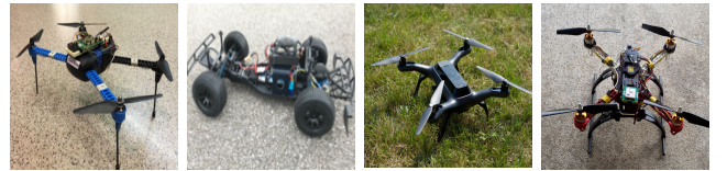
Figure 13: Real RVs in evaluation: 3DR IRIS+, Erle-Rover, 3DR Solo, Self-built (left to right)
