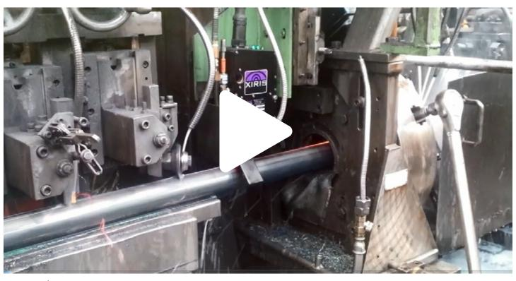
This inline, automated system uses triangulation to generate a 3-D map of the surface to check for weld defects.
