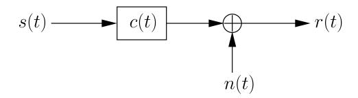
c(t): channel impulse response; \*: linear convolution
