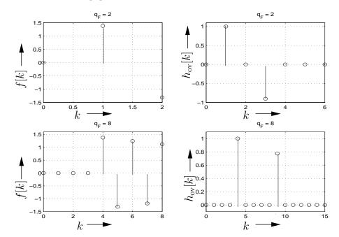
We observe that the residual interference is larger for shorter equalizer filter lengths and increases as the root of H(z) approaches the unit circle.
