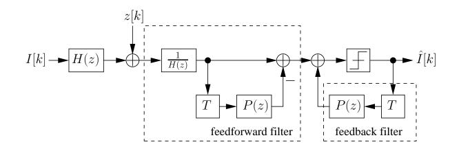
The above structure consists of two filters. A feedforward filter whose input is the channel output signal  $r_b[k]$  and a feedback filter that feeds back previous decisions  $\hat{I}[k-m]$ ,  $m \ge 1$ . An equalization scheme with this structure is referred to as decision-feedback equalization (DFE). We have shown that the DFE structure can be obtained in a natural way from linear equalization and noise prediction.
