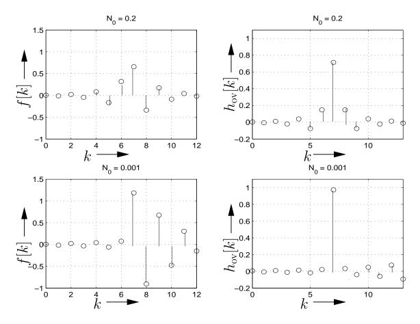
We observe that the residual ISI in  $h_{ov}[k]$  is smaller for the smaller noise variance, since the MMSE filter approaches the ZF filter for  $N_0 \rightarrow 0$ . Also the bias decreases with decreasing noise variance, i.e.,  $h_{ov}[k_0]$  approaches 1.
