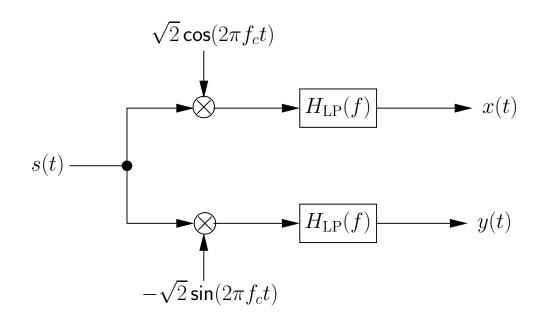
$H_{\rm LP}(f)$  is a lowpass filter. With cut-off frequency  $f_{\rm LP}$ ,  $f_0 \leq f_{\rm LP} \leq 2f_c - f_0$ . The above structure is usually used in practice to transform a passband signal into (complex) baseband.
