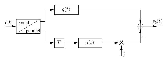
Although the equivalence between MSK and OQPSK only holds for the special g(t) given above, in practice often other transmit pulse shapes are employed for OQPSK. In that case, OQPSK does not have a constant envelope but the variation of the envelope is still smaller than in case of conventional QPSK.
