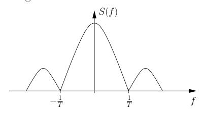
The large side lobes can be avoided by changing the *carrier* frequency smoothly. The resulting signal has a continuous phase.
