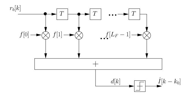
Because of the finite filter length, a complete elimination of ISI is in general not possible.
