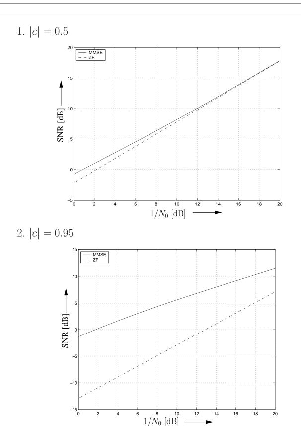
As expected, for high input SNRs (small noise variances), the (output) SNR for ZF equalization approaches that for MMSE equalization. For larger noise variances, however, MMSE equalization yields a significantly higher SNR, especially if H(z) has zeros close to the unit circle.
