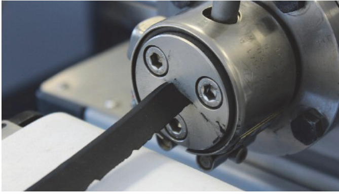
Fig. 2: Extruded Garvey die profile.
