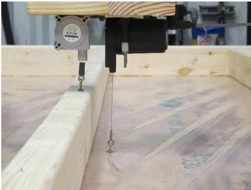
Figure 4 - 2. Installation of two string potentiometers to wood framing member and sheathing. The relative displacement of sheathing under suction pressure is obtained as difference of the two measurements.
