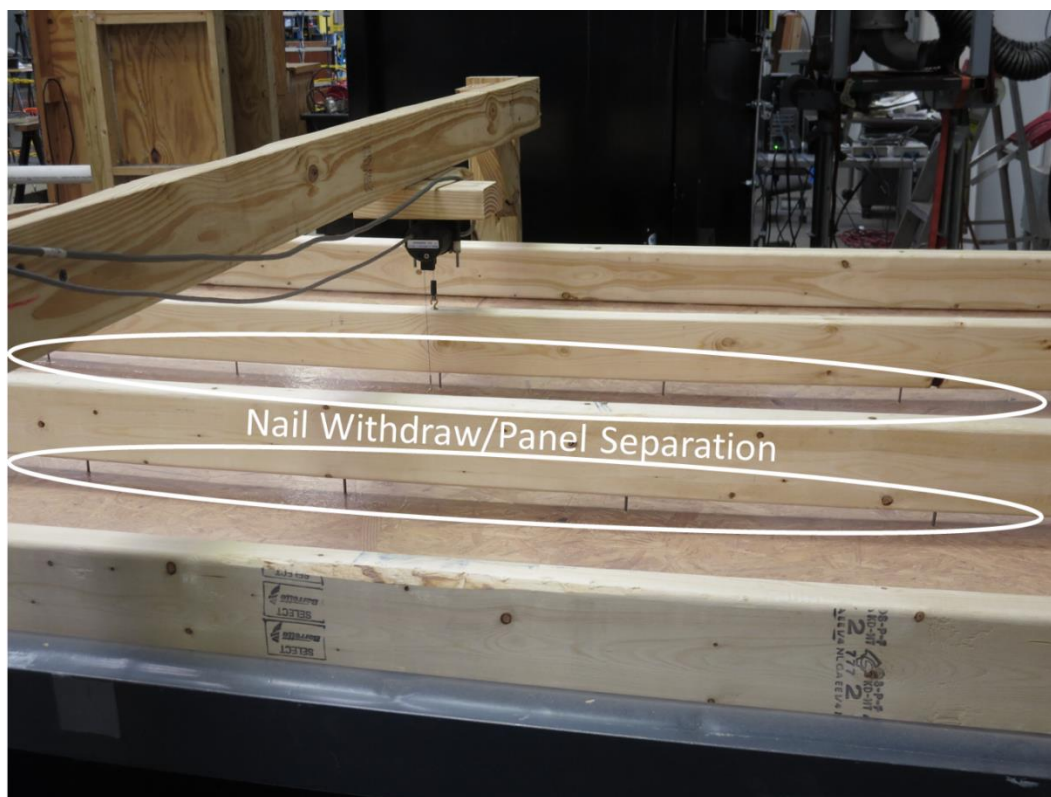
Figure 5 - 1. View of wall panel during testing. The OSB sheathing is pulled away from framing members, with maximum displacements observed at the two middle studs. Initial separation of OSB at both center studs at the same time. OSB test 7.
