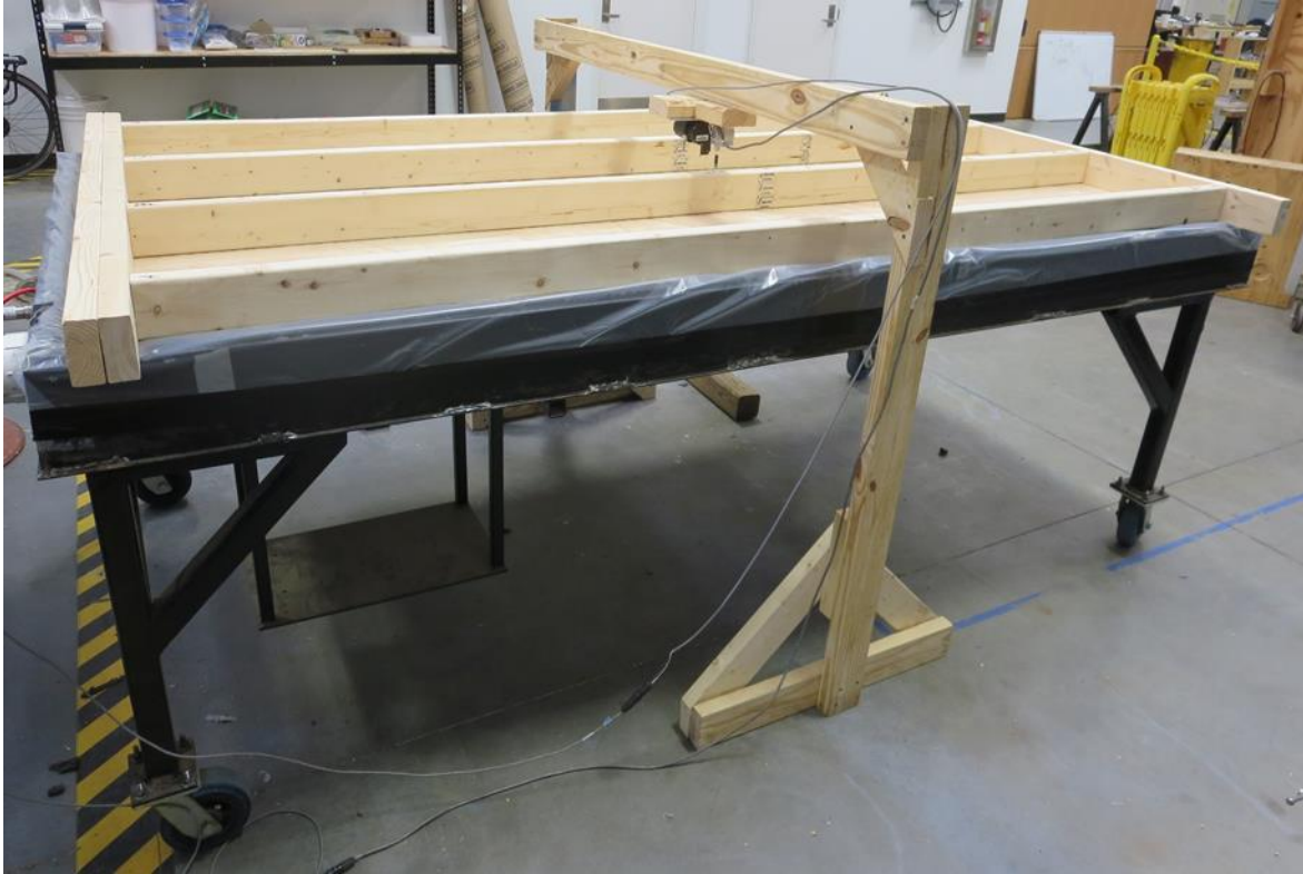
Figure 4 - 1. Test setup for wall tests – wood wall sample installed on steel test chamber. The plastic sheathing draped over sides of steel chamber was placed between sheathing and wood framing and the edges are taped to chamber wall creating air-tight seal.
