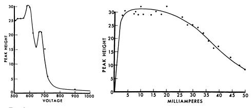
Fig. 2 (left). Effect of varying voltage to photomultiplier tube at optimum gain. Zero adjustment was made using gain control for each determination. Milliamps to hollow cathode = 20. Fig. 3 (right). Effect of varying current to hollow cathode lamp.
