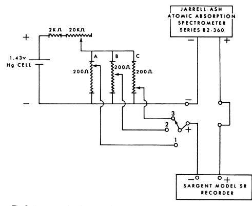
Fig. 1. Zero suppression circuit for adapting 10 mv recorder to atomic absorption spectroscopy. Variable resistances (A, B, and C) are adjusted so that bucking EMF is 5, 8, and 9 mv given a scale expansion of  $\times 2$ ,  $\times 5$ , and  $\times 10$ , respectively.
