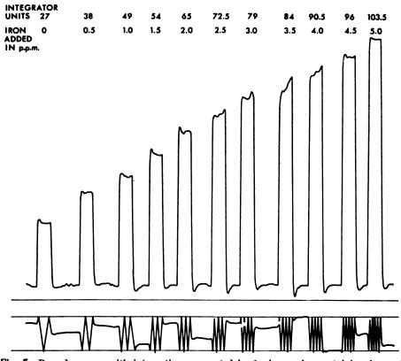
Fig. 5. Recorder curve with integrations generated by 1-ml. samples containing increasing increasing increments of iron.
