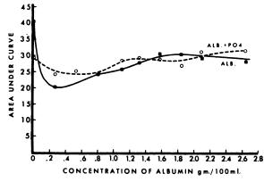
Fig. 8. Effect of increasing concentrations of albumin and phosphate on 200  $\mu$ g./100 ml. iron standard.
