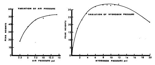
Fig. 4. Effect of varying hydrogen and air pressures. At left, hydrogen pressure is 8 psi. At right, air pressure is 7.0 psi.
