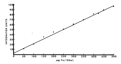
Fig. 9. Standard iron curve. Standards prepared in 6 gm./100 ml. iron-free albumin solution.
