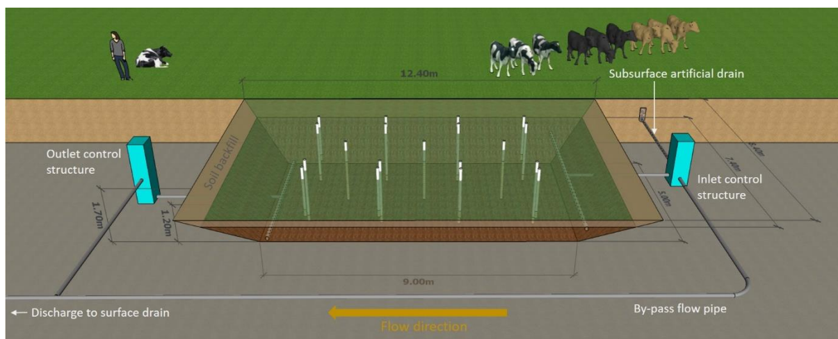
Figure 1 Schematic of the Tātuanui woodchip bioreactor showing the main components of the bioreactor and the monitoring wells from which water was drawn for high-frequency measurements of nitrate. Flow direction is from right to left.
