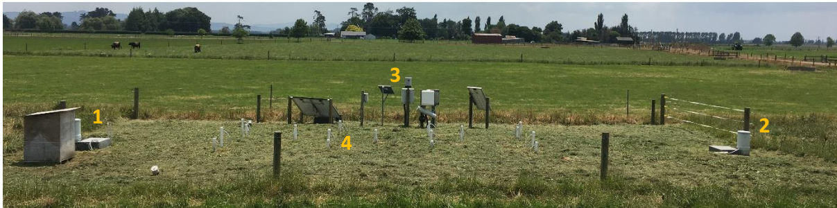
Figure 2 Photo of the completed installation of the woodchip bioreactor showing the main components: (1) inlet control structure with auto sampler and stilling well, (2) outlet control structure with auto sampler and stilling well, (3) multiplex sampling system and optical sensor, rain gauge, solar panel, and control panels for the instruments, and (4) monitoring wells. Flow direction is from left to right.
