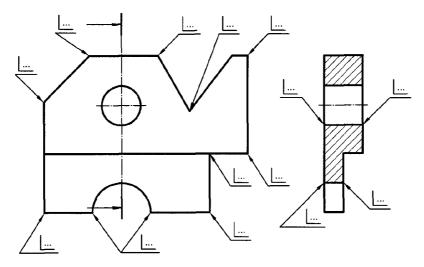
Figure 14 — States of edge vertical to the projection plane and of a feature
