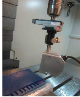
Fig. 8: Measurements taken by laser displacement sensor.
