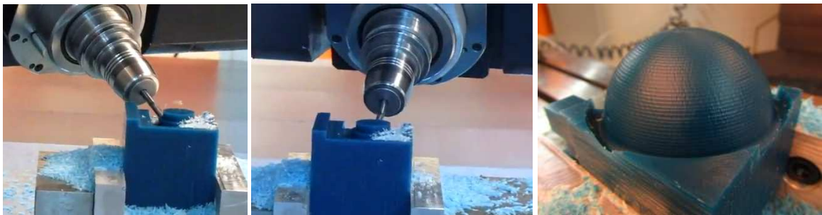
Fig. 5: Using NX Post processor to drive Fryer 5X machining center to make a wax part.
