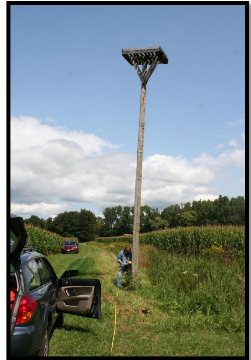
Figure 5: Potential obstacle can also act as a ground control point. This osprey nest tower that is just off planned flight lines was located with GPS.
