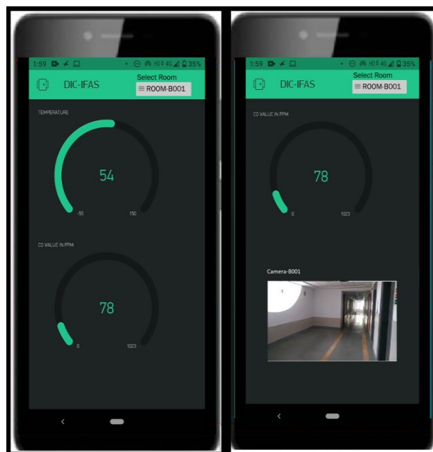
Figure 8. Live information on fire status in mobile with a particular address of room and building.
