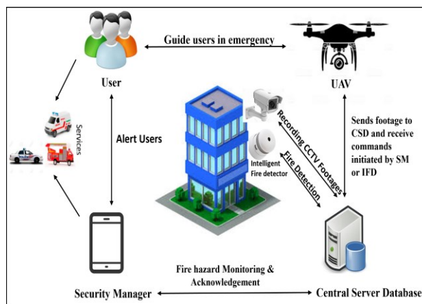
Figure 1. UAV based fire alarm system
