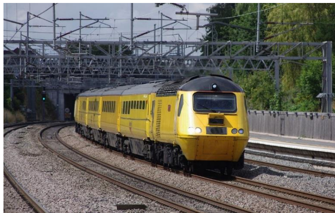
Figure 6: The New Measurement Train
