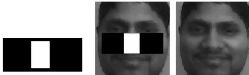
Figure 2: Example of a Haar feature used to detect eyes and bridge of nose.
