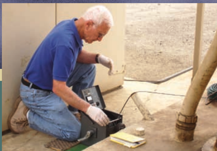
Measuring depth to water in a well.
