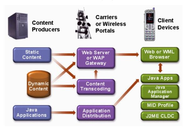
At the top left of the figure, you have content that comes out of simple, static files. Dynamic content is also generated in application servers and Web servers, largely based upon information extracted from a database and being modified dynamically using Java Servlets, Enterprise JavaBeans (EJBs), or other server-side technologies.
