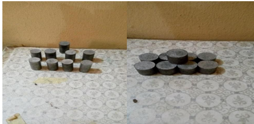
Figure 3: Green compact specimen
