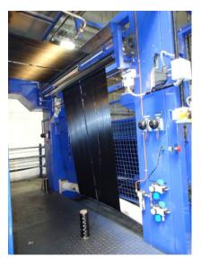
Oxidized sample fed through commercial line furnace; carbon fiber wound using commercial winder
