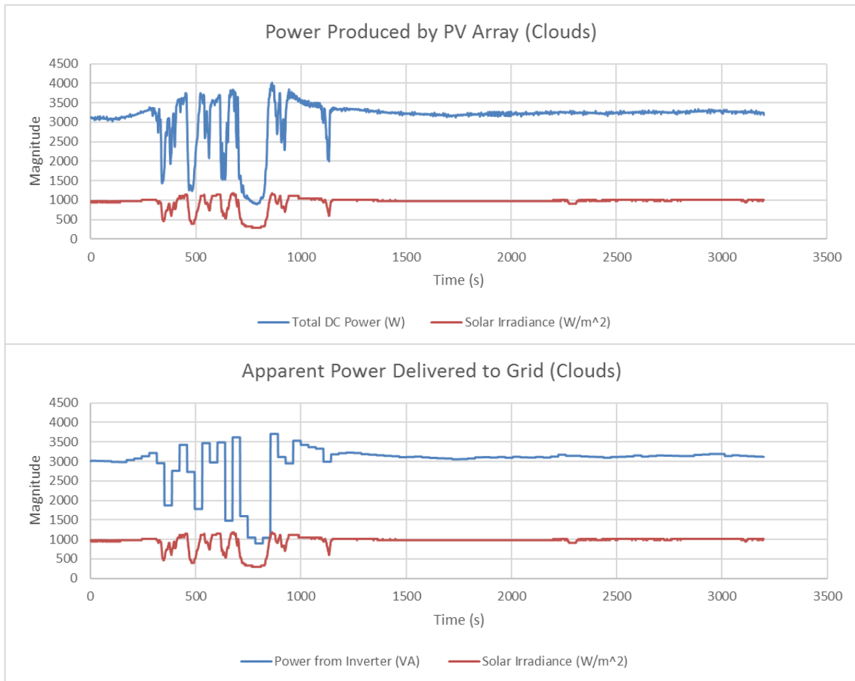
Figure 34: Power Produced by PV Array and Apparent Power Delivered to Utility Grid During Intermittent Cloud Cover
