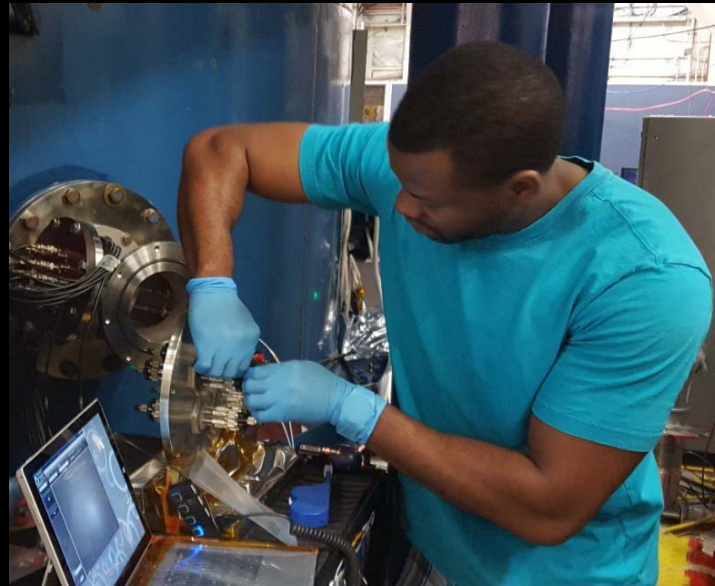
Eleanya Onuma installs vacuum feedthroughs
