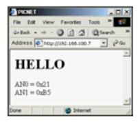
☐ Turn the potentiometer on the prototyping board and refresh the page to change what is displayed on the webpage. While a web browser is connected to the prototyping board, the IP address of the web browser will be displayed on the second line of the LCD. If no browser is connected, it should say 'Listening'.
