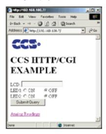
The website uses an HTML input form to change the data displayed on the LCD and to change the status of the two LEDs. Click on the "Analog Readings" link to go to another page on the prototyping board server that displays the current ADC reading of AN0.
