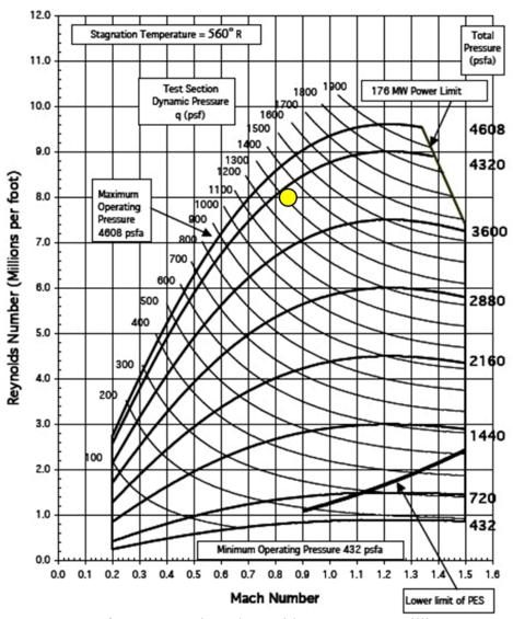
Figure 20: Ames 11-ft WT Operating Chart with CRM Rn<sub>c</sub>=5 million Test Condition.
