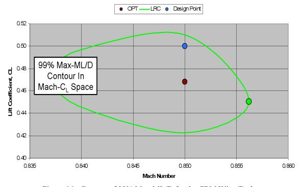
Figure 16: Contour of 99% Max-ML/D for the CRM Wing/Body.
