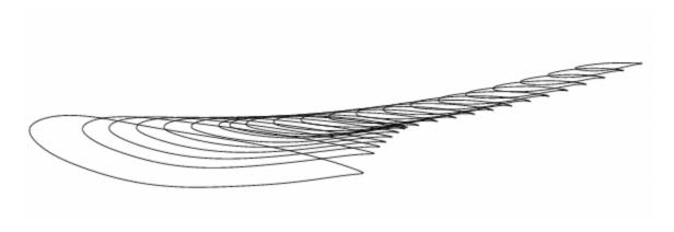
Figure 2: Airfoil Stack for the CRM Wing.
