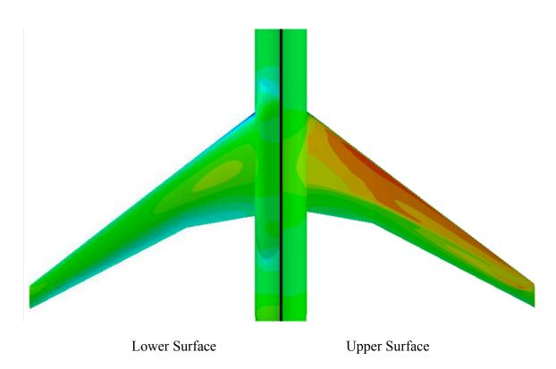
Figure 12: OVERFLOW Isobars of the CRM Wing/Body at the Design Point.
