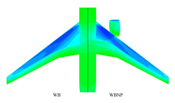
Figure 17: TRANAIR Results of Nacelle-Pylon Effect on Wing Upper-Surface Isobars.
