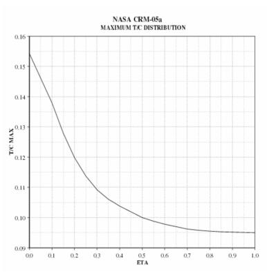
Figure 3: Non-Dimensional Thickness Distribution of the CRM Wing.
