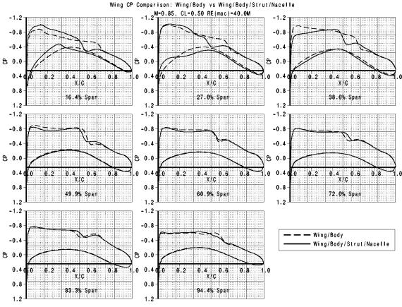
Figure 18: TRANAIR Results of Nacelle-Pylon Effect on CRM Wing Pressures.
