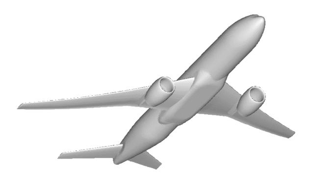
Figure 9: CRM Wing/Body/Nacelle/Pylon/Horizontal-Tail Configuration.
