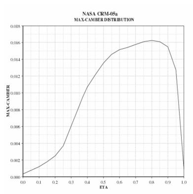
Figure 5: Max-Camber Distribution of the CRM Wing.
