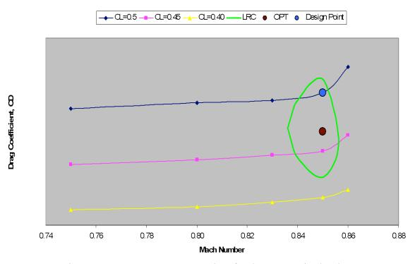
Figure 15: OVERFLOW Drag Rises for the CRM Wing/Body.
