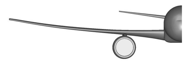
Figure 10: Front View of the CRM showing the Large-Diameter Flow-Through Nacelle.
