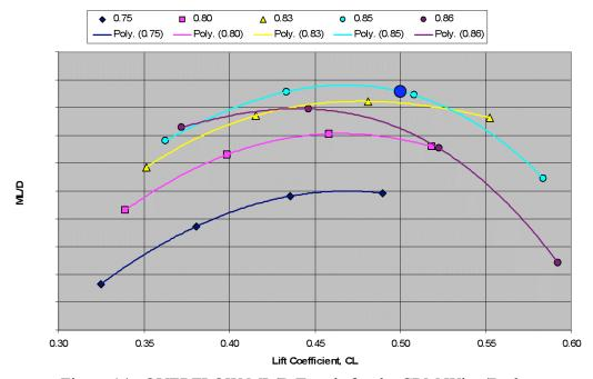
Figure 14: OVERFLOW ML/D Trends for the CRM Wing/Body.
