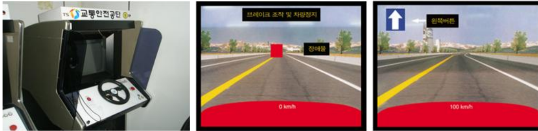
Figure 1 Driving precision aptitude test device and sensory motor factors
