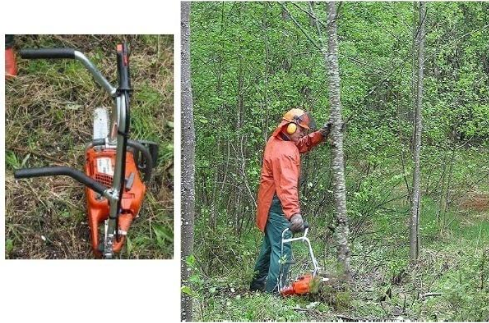
Fig.43. Chainsaw with special handle used in Finland for manual felling (Sikanen, Röser, & Asikainen, 2005).
