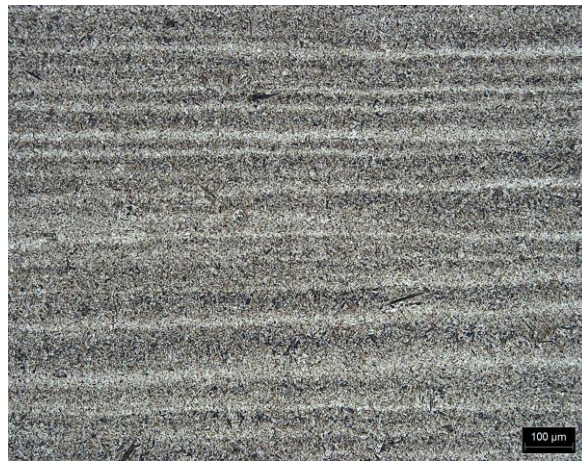
Figure 20. Banded structure etched in 2% Nital.
