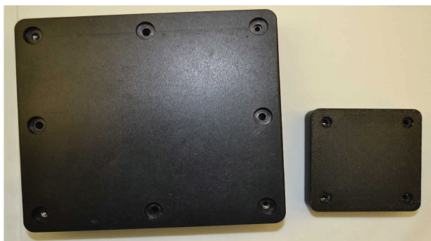
Figure 1. The mLCCE (right) is 80% smaller than the LCCE (left).
