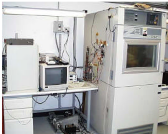
Figure 2. Sperry Sun HALT Equipment
