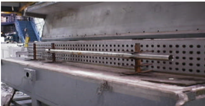
Figure 6. Sperry Sun MWD Tool Being Prepared for Oven Test
