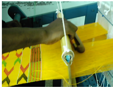
Figure 14b: Weaving in progress ready for the beating up
