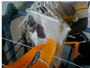
Figure 12b: Weaver engaged in the heddling process
