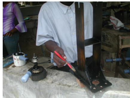
Figure 7b: Painting metal component with oil paint
