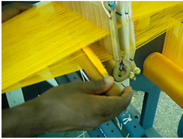
Figure 14a: Created shed ready for weaving
