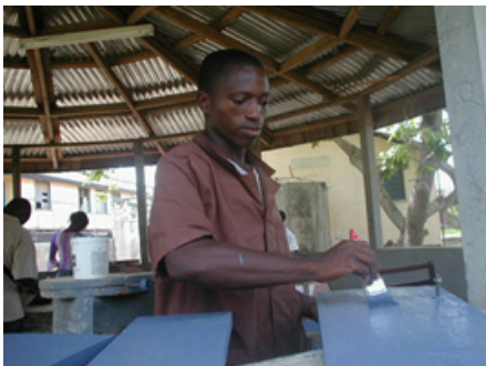
Figure 7a: Painting the frame of the loom with acrylic paint
