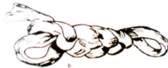
Figure 9b: The chain stitched warped yarn
