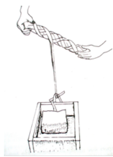
Figure 11: Beaming by the box method originally used as the warping stone ( Tweso )
