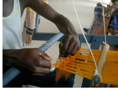
Figure 13b: Securing the warps to the cloth roller
