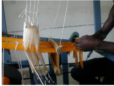
Figure 13a: Taunting the warp sheet to the cloth Roller
