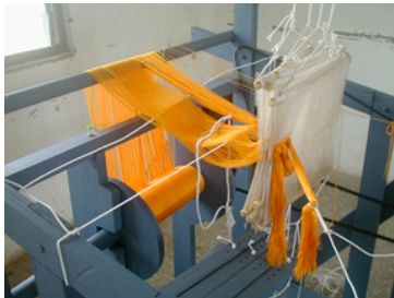
Figure 12a: Beamed warp ready for heddling
