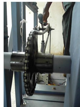
Figure 15b: Tautening mechanism displayed in the sitting position
