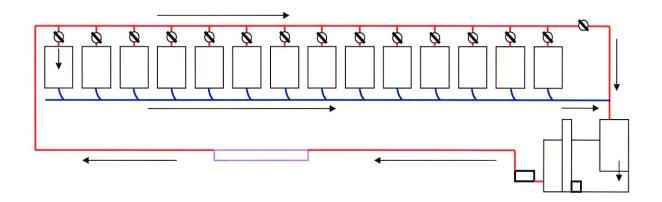
Figure 2. Schematic diagram of rearing tank (side view). (A) return line, (B) divider (500micron netting), (C) air diffuser, (D) drain line. Arrows indicate direction of water flow.
