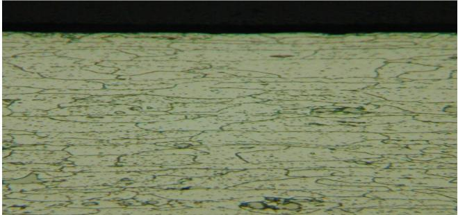
FIGURE 3 Microstructure of 5083-H321 doublet plate, as received. Etched, 550X
