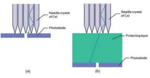
Fig.1 Schematic cross section of scinttilator and TFT-panel. (a) AeroDR, (b) Conventional DR.
