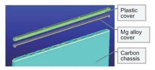
(a) Construction of chassis edge
