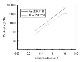
Fig.3 Digital characteristic curves of AeroDR and PLAUDR.
