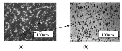
Fig.1. SEM micrographs of (a) Binary and (b) Hybrid MMC.
