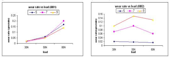
Fig. 2 Effect of load on wear rate of composites for different speeds: 05, 07 and 09m/s.
