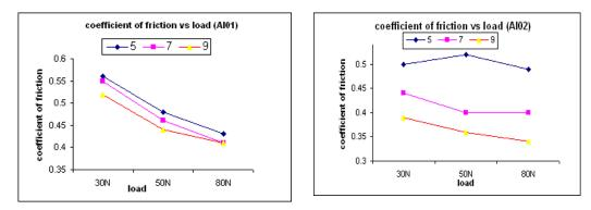
Fig. 3 Effect of load on coefficient of friction at different speeds: 05, 07 and 09m/s.
