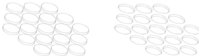
Figure 31. Isometric perspective drawing of embossed pattern for origin (left) and debossed pattern for insertion (right).
