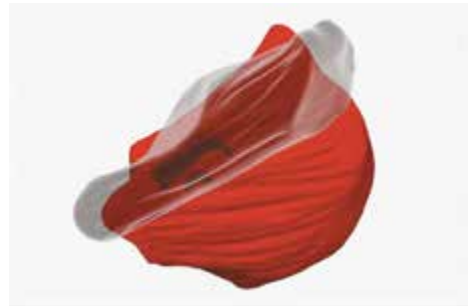
Figure 28. Press fitting with pocket for magnet to attach pterygoids to on another.
