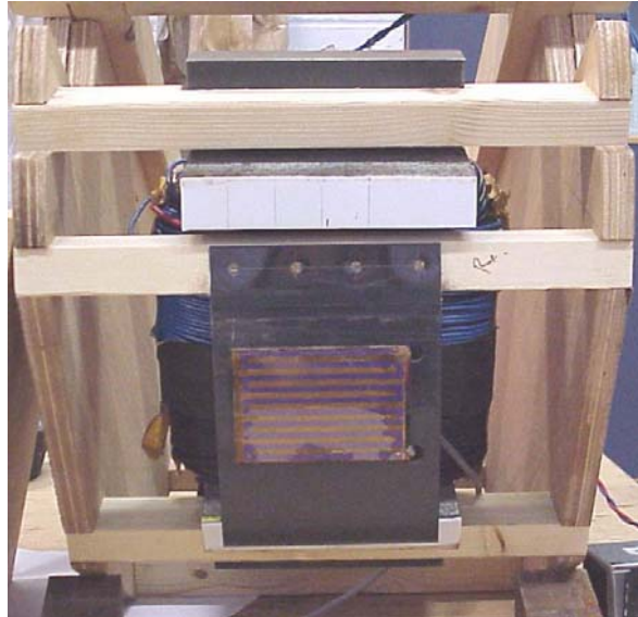
Figure 15 Side view of the SV1 carriage showing the meander line (ML) coil and circumferential biasing electromagnet in position.
