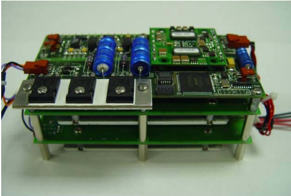
Figure 21 Mule prototype transmitter control (top board), driving stacked above positive and negative high voltage supply boards
