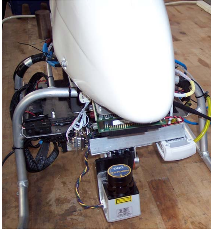
Figure 3.2. Mounting of Obstacle Detection System Components on the SR-20.
