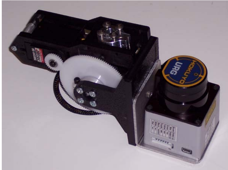
Figure 2.5. Servomotor, Sensor Mount and LIDAR Sensor
