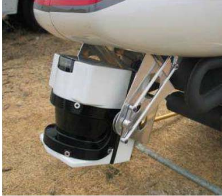
Figure 1.5. Sick Scanning LIDAR Unit Mounted on a Berkley R-Max UAV [10]
