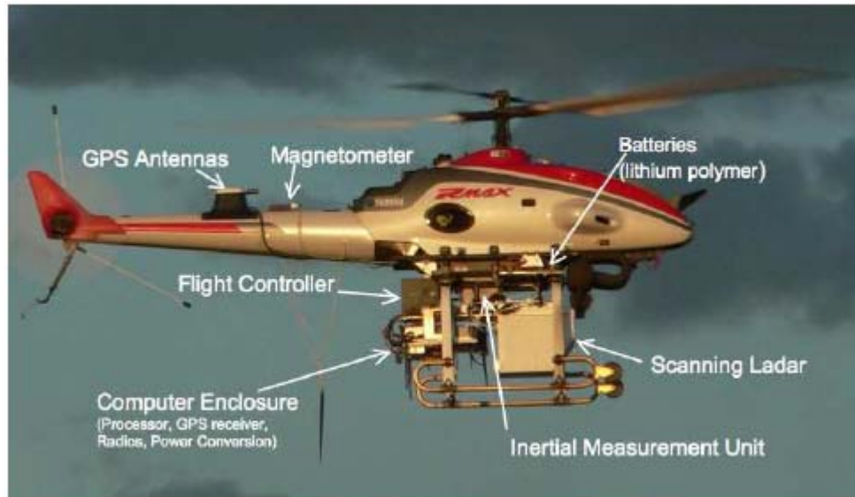
Figure 1.6. CMU R-Max with Fibertek Inc. Scanning LIDAR Onboard [11]
