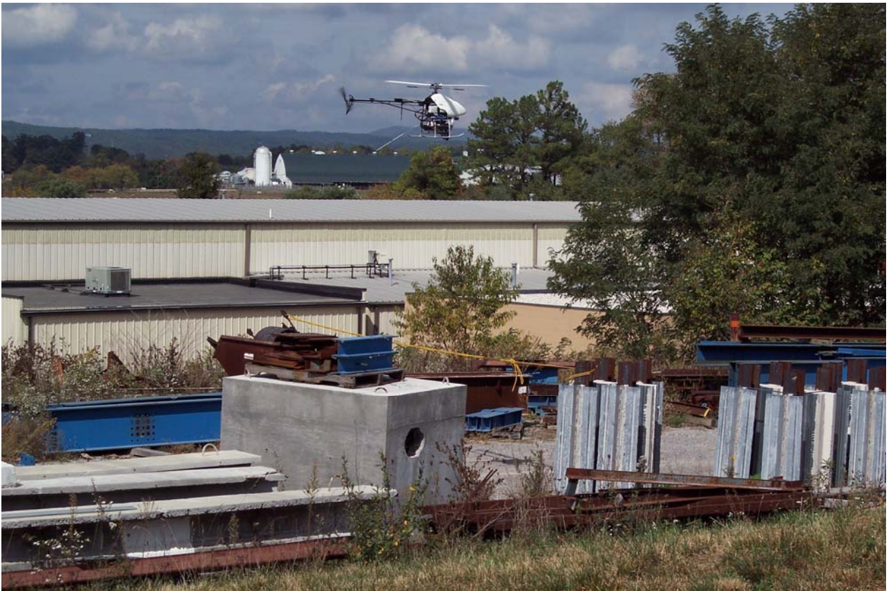
Figure 4.10. Flight test of the SR-20 Using the Obstacle Detection Payload above Obstacles
