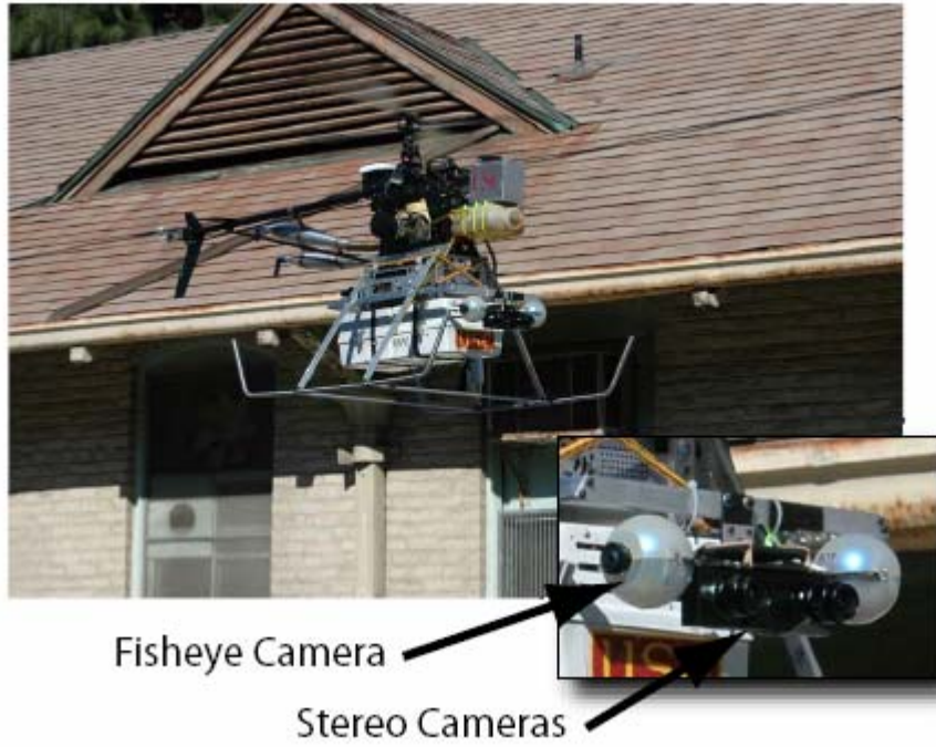
Figure 1.7. USC Avatar platform with Vision System [12]
