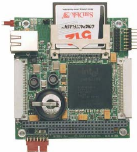
Figure 2.2. SBC1586 PC/104 Single Board Computer [14]
