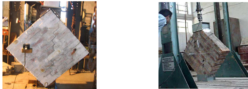
Fig. 5: Evaluation of diagonal strength of masonry panel, from [29] (left) and test conducted at the UET Peshawar (right).
