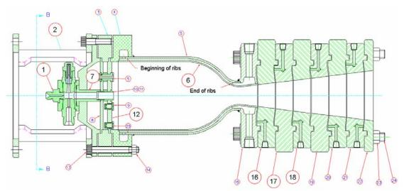
Figure 3: General drawing in longitudinal cut of thrust chamber.
