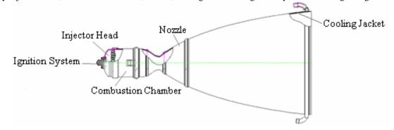
Figure 1: Thrust chamber
