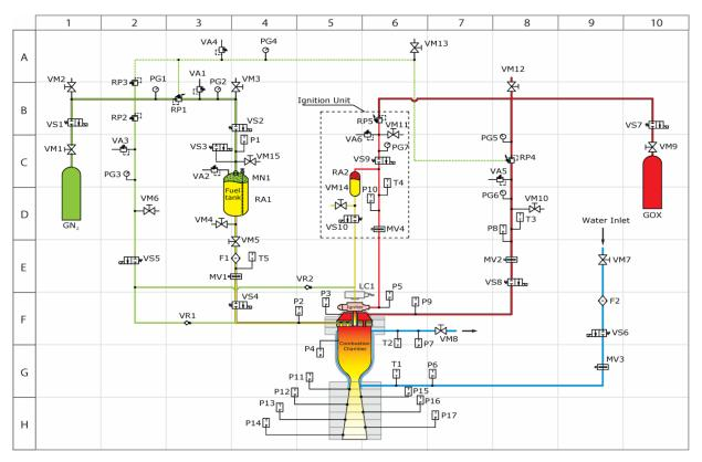
Figure 5: Hydropneumatic scheme.
