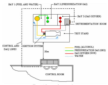
Figure 6: Layout of test complex.
