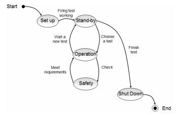
Figure 8: Test Stand State Diagram.
