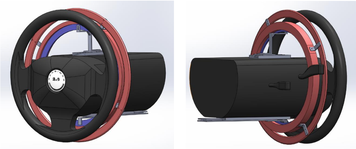
Figure 17 Double Rail System
