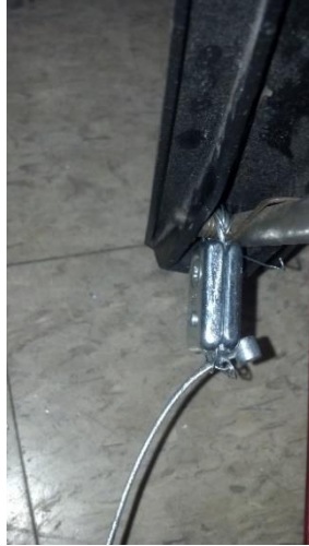
Figure 40 Attaching the Clutch Cable to the Clutch Pedal
